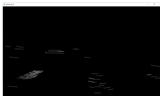
Figure 16: crosstie edge point set recognizing result
