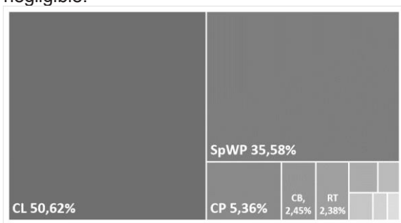
Fig. 13. SpW router components LUT usage.
