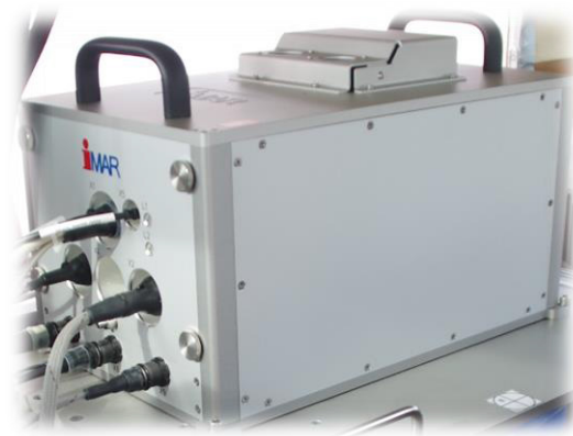
Figure 21: iMAR's iCORUS Gravimeter system
