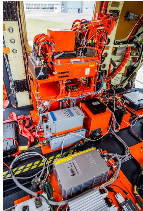
Figure 8: Example of iNAT-RQT integration in H145 helicopter at Airbus Helicopters.
