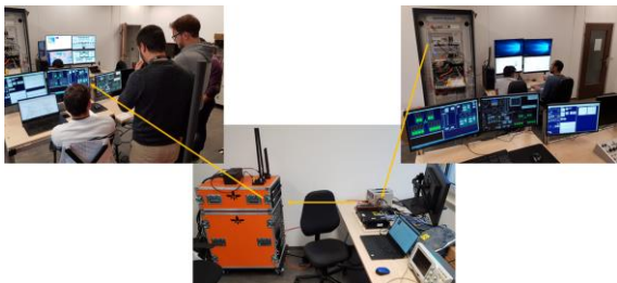
Fig. 9. Lilium FTI SiL and HiL integration tests.
